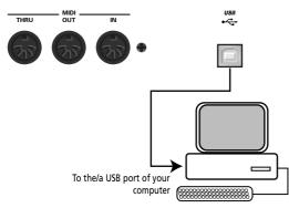
**Note:** Always connect the E-80 directly to your computer or to a powered USB hub.
